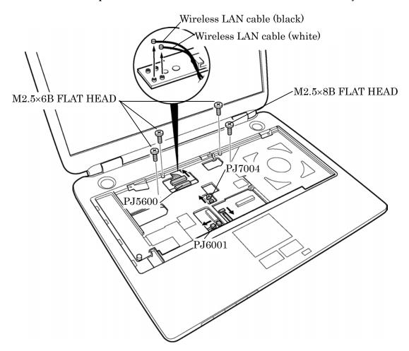
Figure 4-16 Removing the display assembly (2)
